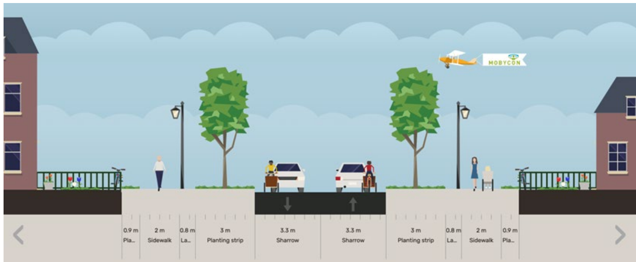
Figure 5-8: Proposed Typical Cross-Section for Local Roads
