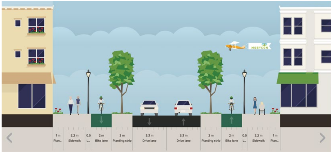
Figure 5-23: Proposed Typical Cross-Section for Collector Roads
