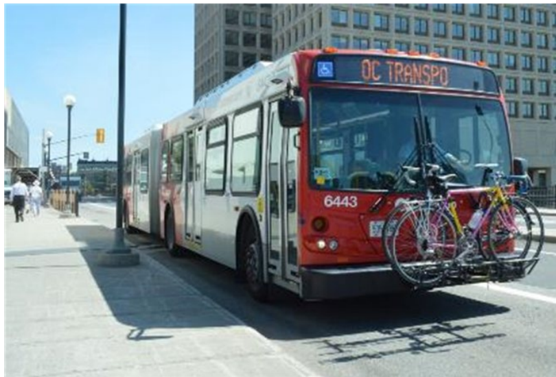
Figure 5-58: Bicycle Racks on Transit Vehicles
